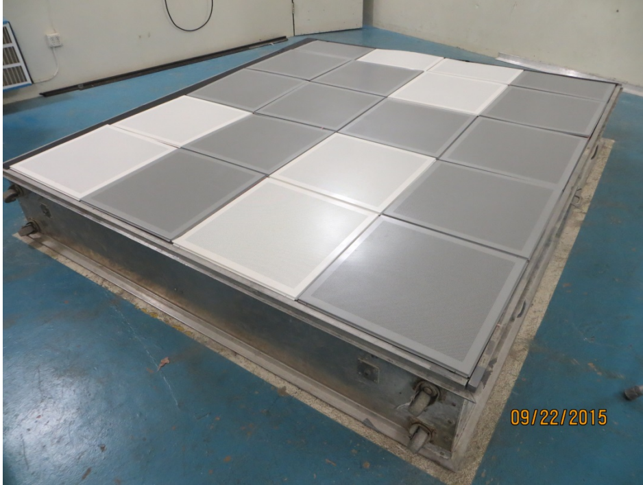
Figure 1 – Specimen mounted in the test chamber.
