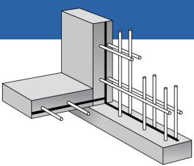
In this cross-section of both horizontal and vertical joints, PENEBAR SW is installed in and along the joint after the first concrete pour and just before the second pour.
