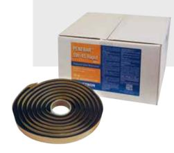
Recommended for non-moving cold joints in building foundations, slabs, retaining walls and storage tanks, PENEBAR SW – 45 Rapid is a fast-acting, concrete joint waterstop designed to expand rapidly when exposed to water.
