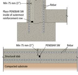
PENEBAR SW is placed in construction joints that have a mandatory 50 mm (2") of concrete coverage.
