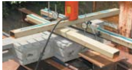
Four-foot lintel tested
