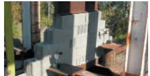
Seven-foot lintel tested up to 20 tons
