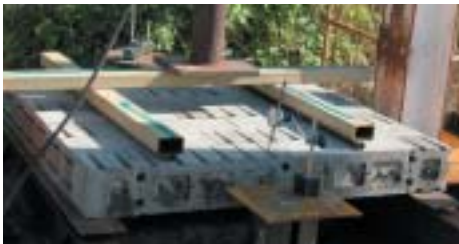
Special wall - all cells filled & two rebars in each cell (Tested to the equivalent of 585 mph wind force)
