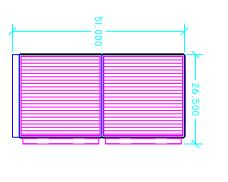
DATE: 01/24/05 CFM: DRWG. NO.: FW2-012405 DRAWN BY: TA/ SHEET TITLE: AZTECH 3500 FW2 MOTOR: DIMENSIONS: SPECIFICATIONS: 51"H X I20" W X 26.5" D 2 HP 208-230/460/3/60 TEFC 3 HP 208-230/3/60 TEFC 2 HP - 4000 CFM 3 HP - 4500 CFM
