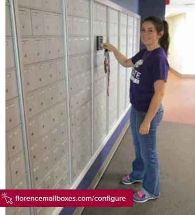
Rear-load mailboxes (1700 series) have an exposed back for easy distribution, so keep in mind during planning that additional space will be necessary for a secure room behind the installation. Access to the room may be restricted and easily accessed using a key keeper (see page 36) with a private lock.
